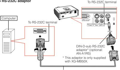
RS-232C serial control cable (cross type, commercially available)
